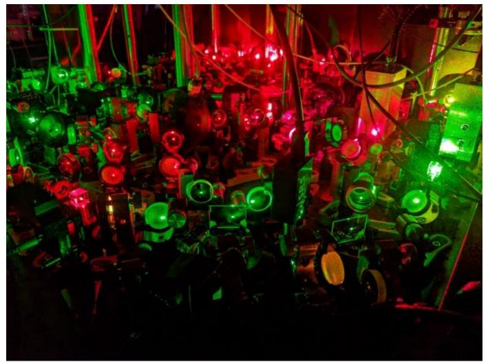
Red light stop: The experiment uses multiple frequencies of light to cool the CaOH atoms to a fraction of a degree above absolute zero. (Courtesy: John Doyle)
