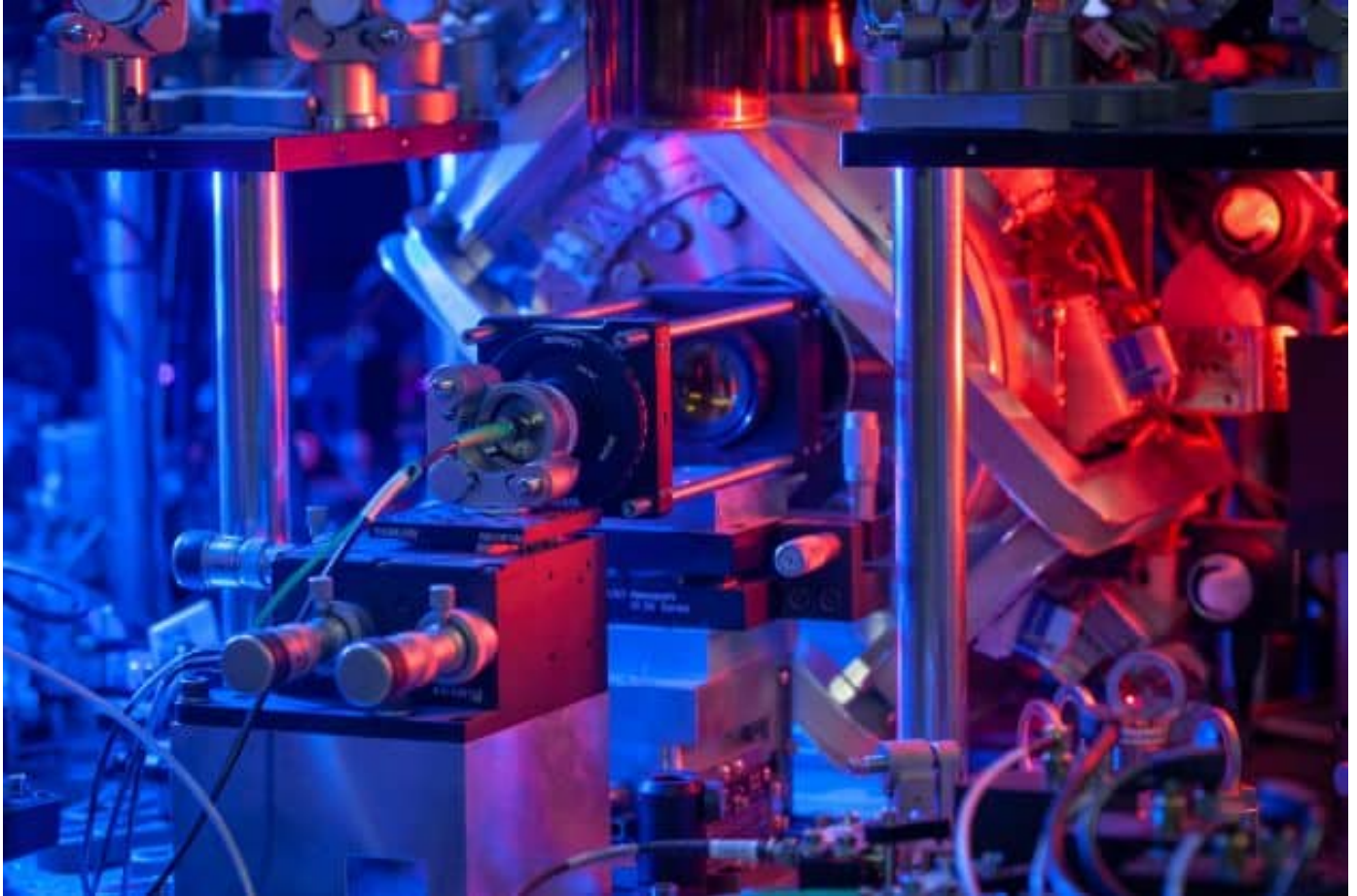
Network node: A vacuum system containing the ion trap used to create the "Bob" node in the Oxford-CEA-Switzerland experiment. (Courtesy: David Nadlinger/University of Oxford)
