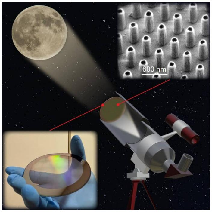
Future telescope: photomontage showing the metalens (bottom left) and part of its microscopic structure (upper right). Also shown is an image of the moon (not taken by the metalens) and an artistic impression showing how the metalens was used in a telescope. (Courtesy: Lidan Zhang et al/ACS Nano Letters)
