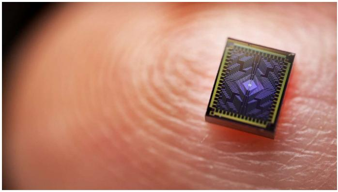
Chip off the old block: Intel's Tunnel Falls chip is based on silicon spin qubits, which are about a million times smaller than other qubit types (Courtesy: Intel Corporation)
