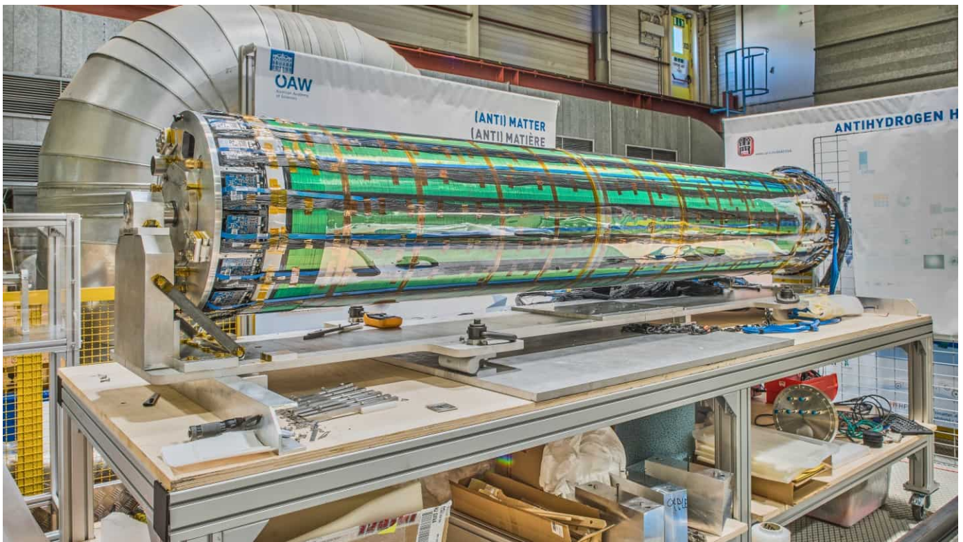
Going down: ALPHA-g's barrel scintillator being assembled at CERN. (Courtesy: CERN)
